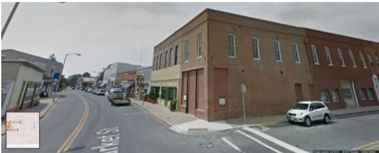
2. Functional, but not fully ADA-compliant - at least 3 feet wide, includes flares and ramps, but not "bubbled," and ramps may be narrower than the rule. No utility poles in sidewalk. This view is Market Street and College Avenue in Onancock. A crosswalk connects two Category 2 sidewalks.
