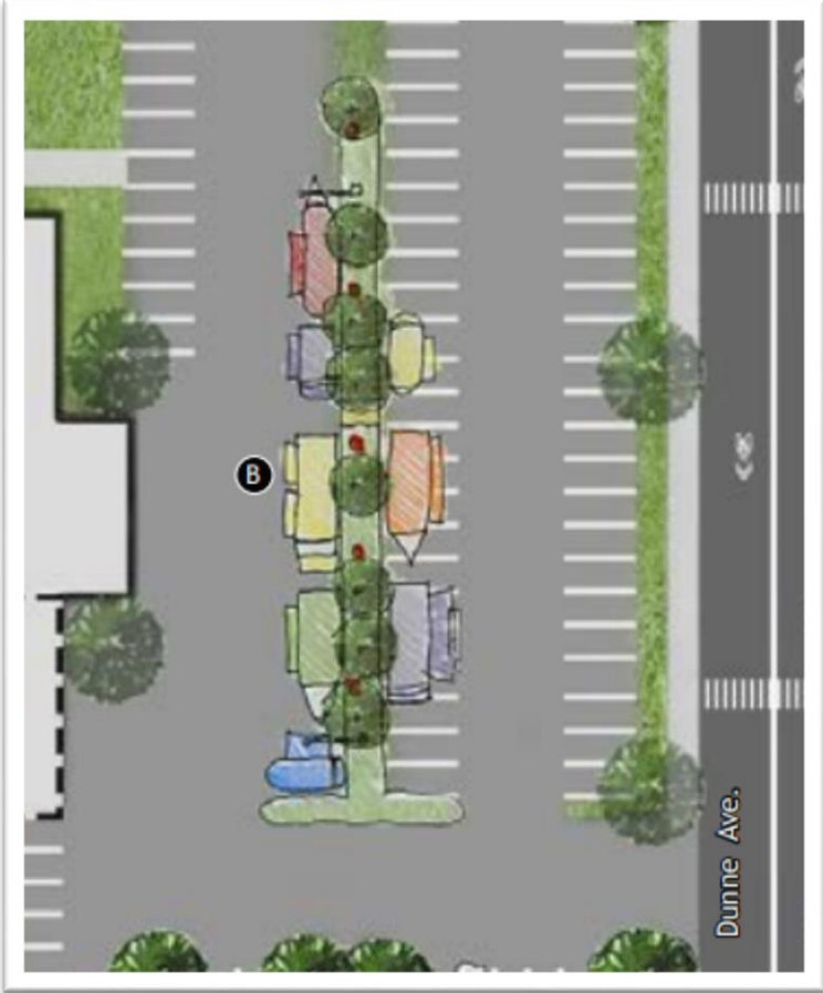
Master Plan for the expansion of the Farmer’s Market including utility bollards to sport food trucks and vendors.
