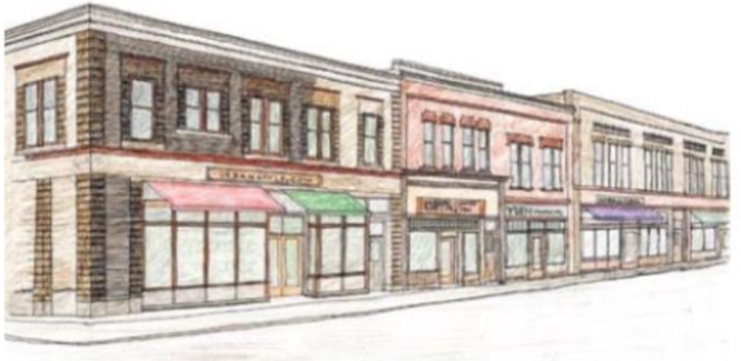
AFTER Removing materials that cover brick and display windows restores the street's rhythm and clearly identifies building entrances.
