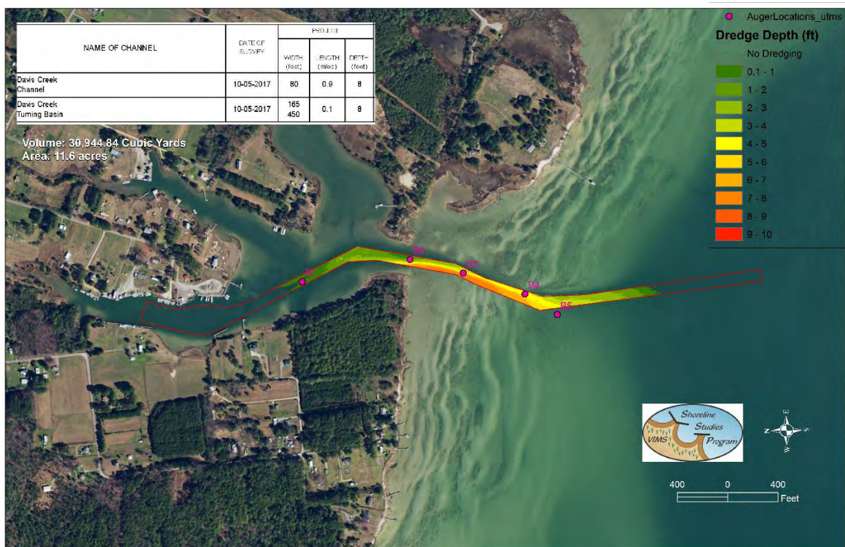
Figure 5-4. Davis Creek channel showing the amount of material that needs to be dredged and the auger sample locations.
