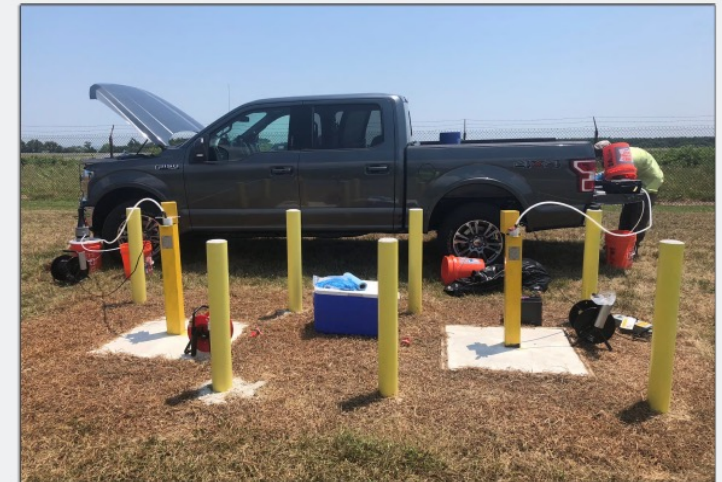
Low-flow sampling of PFAS monitoring well
