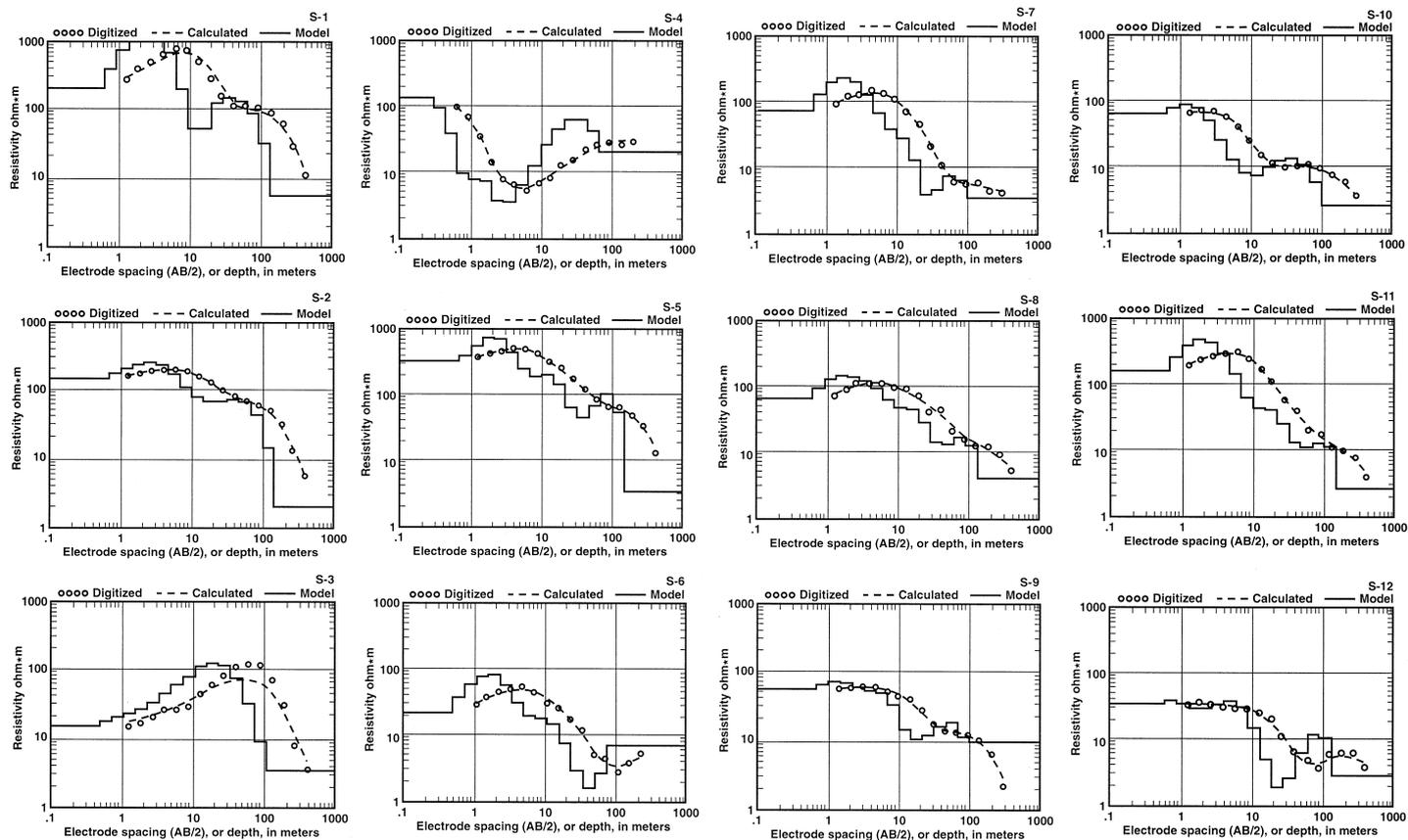
Fig. 5. Presentation of 12 sample soundings. Digitized field curves, circles. Subsurface models, solid lines. Theoretical curves based on models, dashed lines.
