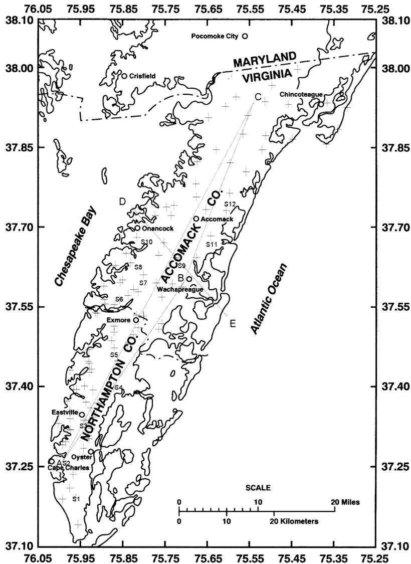
Fig. 4. Central positions of the 111 Schlumberger soundings are marked by +. The results and conclusions of this paper are based on all 111 soundings. Only the details of 12 soundings, marked s1 to s12, are presented in Fig. 5.
